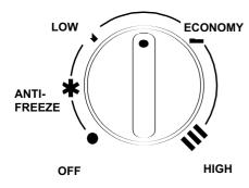
The economy setting "E" will maintain stored water temperature at approximately 60°C. At the "E" setting, the temperature control locates into a set position and a slight resistance will be felt when rotating the temperature control beyond that setting. This measure is to help ensure that higher temperatures are only selected deliberately.
